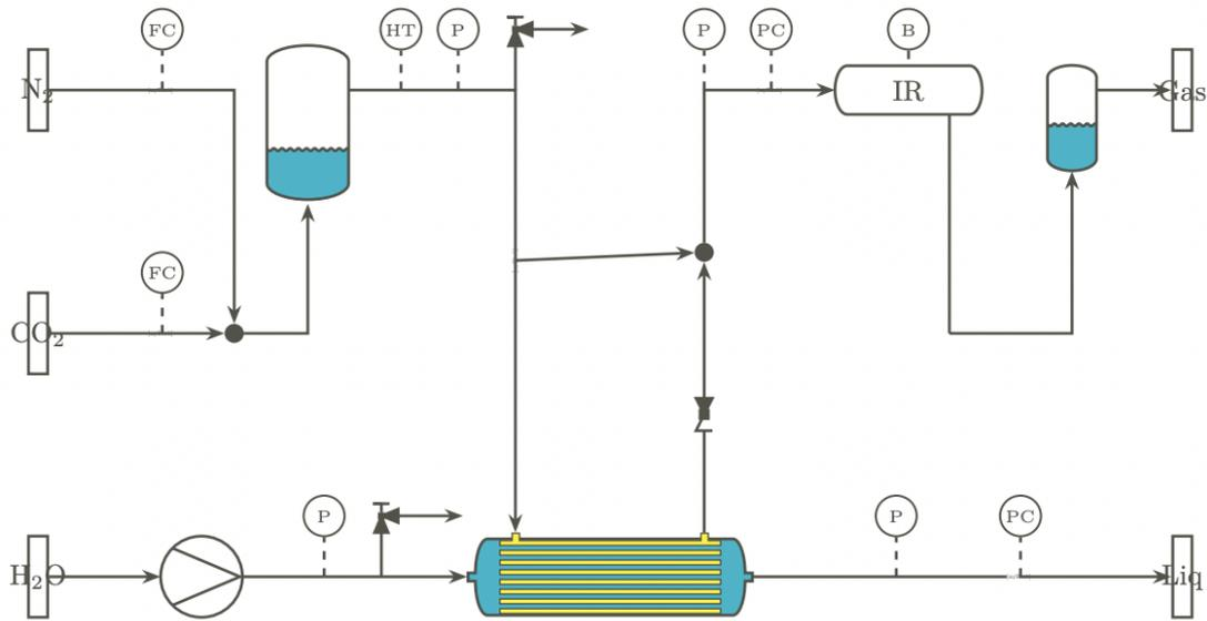
**Figure 3.1:** The experimental setup for the membrane contactor rig<sup>[2]</sup>. F stands for flow, H for humidity, P for pressure, T for temperature and C for control.
