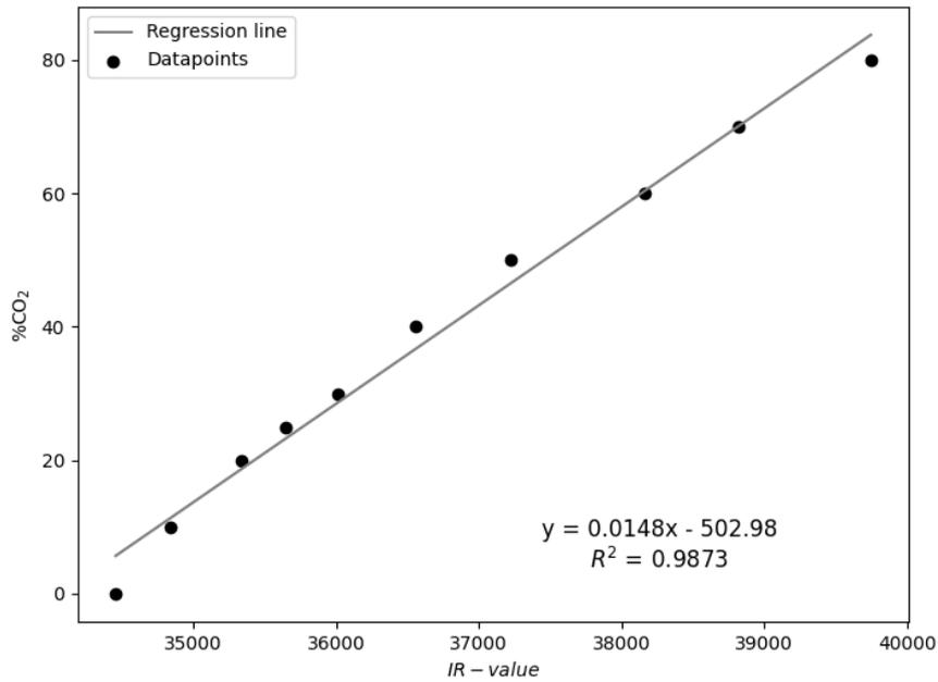
**Figure B.1:** Plot of the linear regression made from the 16-bit values and the concentrations of CO<sub>2</sub> in Table B.2.
