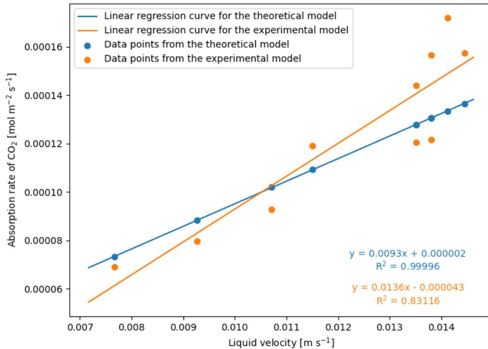
Figure 4.1: Plot of the results with linear regression lines for the theoretical and experimental model.
