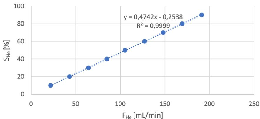
Figur B.6:  $S_{He}$  as a function of  $F_{He}$ , plotted with values from calibration data.<sup>[2]</sup>
