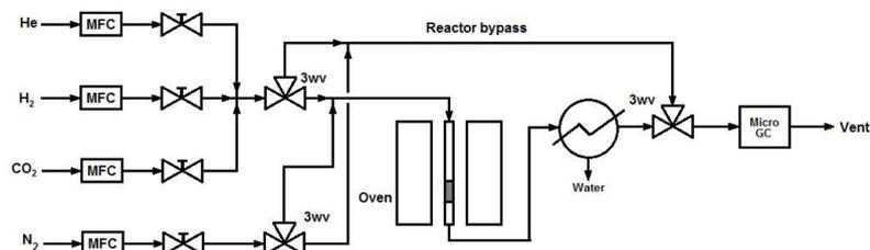
Figur 2.1: Simplified flow chart of the experiment and the testing apparatus used. Mass-flow controllers (MFC), three-way valves (3wv) and gas chromatograph (GC).
