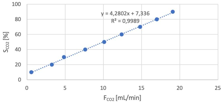
Figure B.3:  $S_{CO_2}$  as a function of  $F_{CO_2}$ , plotted with values from calibration data.<sup>[2]</sup>
