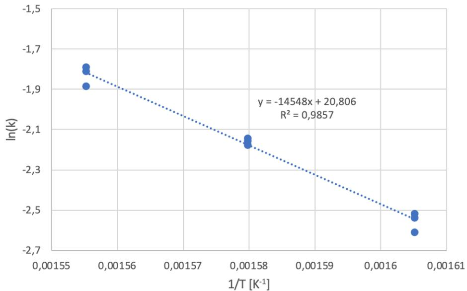
Figur 3.4:  $\ln k$  as a function of  $\frac{1}{T}$  [ $\text{K}^{-1}$ ] for steps 3-5.
