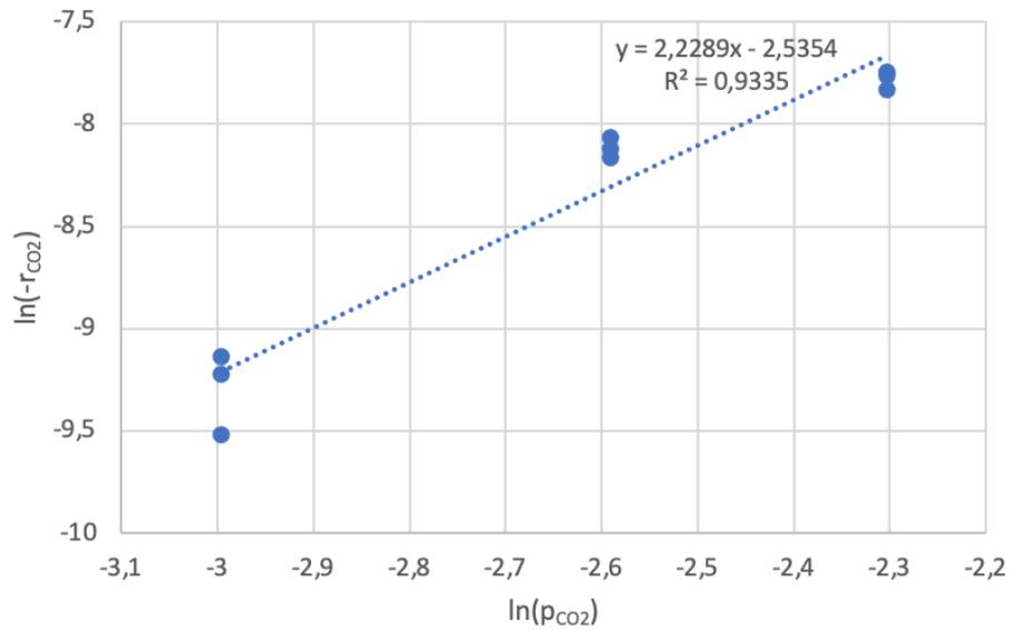
Figur 3.3:  $\ln(-r_{\text{CO}_2})$  as a function of  $\ln(p_{\text{CO}_2})$  for steps 1-3.
