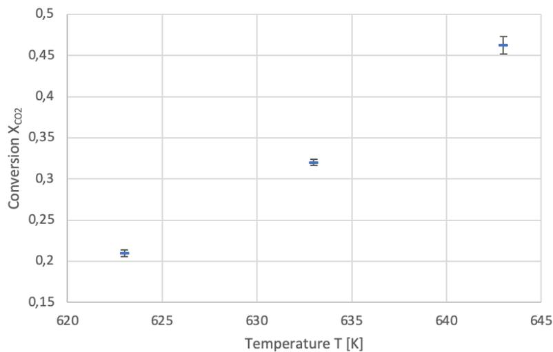
Figur 3.2: The conversion  $X_{CO_2}$  as a function of temperature T [K] for steps 3-5.
