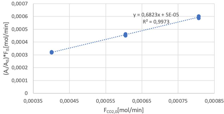
Figur B.1: The calibration curve used to find  $RRF_i$
