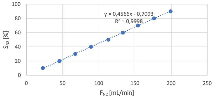
Figur B.5:  $S_{N_2}$  as a function of  $F_{N_2}$ , plotted with values from calibration data.<sup>[2]</sup>
