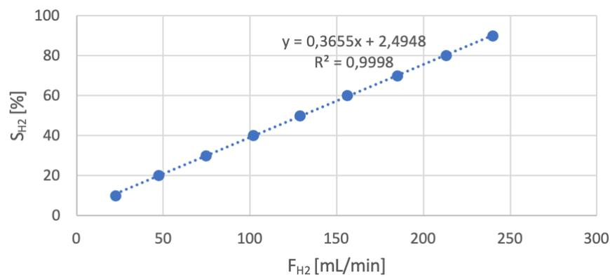
Figure B.4:  $S_{H_2}$  as a function of  $F_{H_2}$ , plotted with values from calibration data.<sup>[2]</sup>
